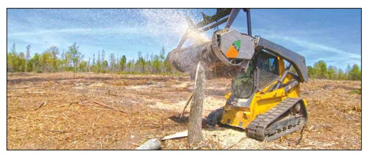
The Sonic System from FAE increases productivity of its excavator-mounted mulchers up to 30% by increasing torque and reducing recovery time from stalling.
