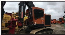
2014 Barko 240 Feller Buncher SN: 23625, approx. 859 hrs., Tracked Feller Buncher w/Quadco Hot Saw (18C)
